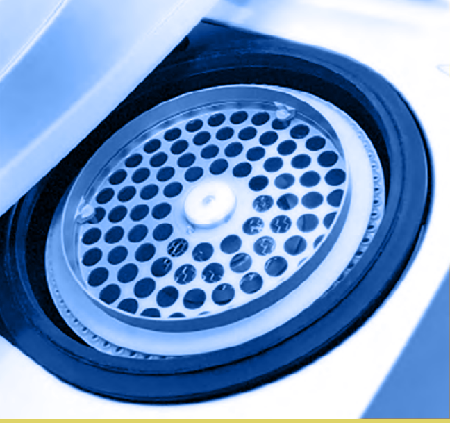
Sapphire Rotor Disc 72, installed in a QiaGen Rotor-Gene Q instrument
